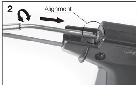
Place the new cartridge in the solder feed handle. **Important:** It is essential to insert the cartridge till the end for a good connection. Use the mark
