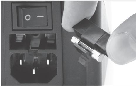
Remove the fuse by pulling the black cap. Help yourself with a lever tool if necessary.
