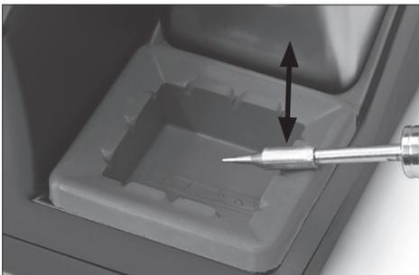
Tap smoothly the cartridge on the wiper profile to remove the excess of solder
