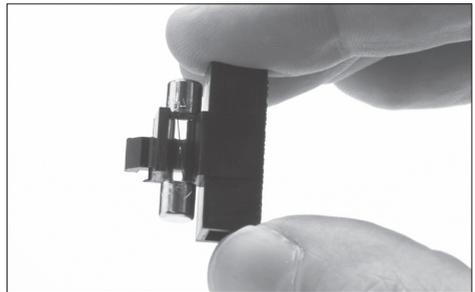
Place the new fuse into the holder by pushing and enter it again into the station.
