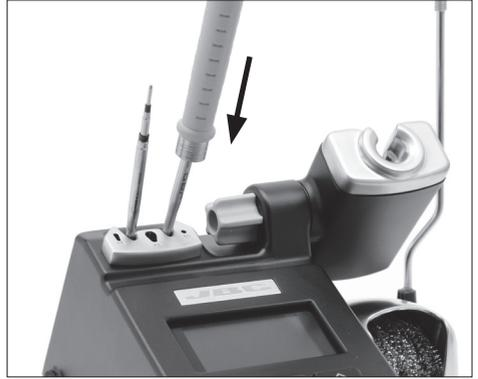
Place the handpiece on top of the new cartridge, press it slightly down and remove the handpiece from the extractor.
