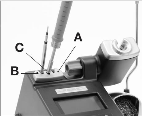
Press the cartridge into the opening A, B or C:
