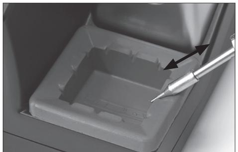
Use the slots to wipe any possible particle stuck on the tip
