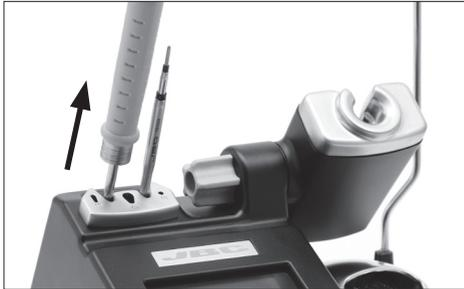
Place the handpiece in the extractor and remove the cartridge.
