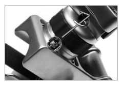
**5.** Fit the new assembly in the Rework Arm and screw it with the allen key using the four supplied screws.
