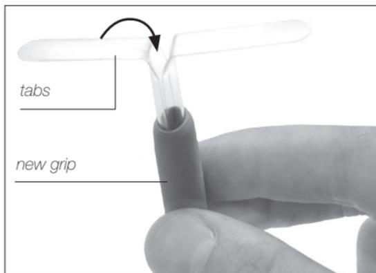
2. Push the grip with the tabs onto the handle.
