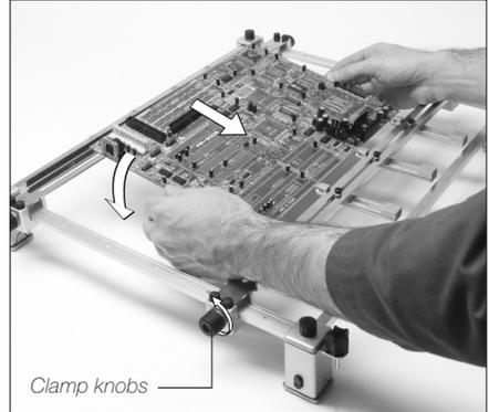
Position it and tighten the sliding guide knobs.
