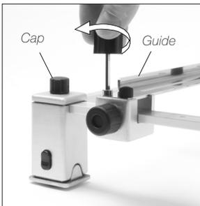
1. Remove both guides by untightening the 8 screws.
