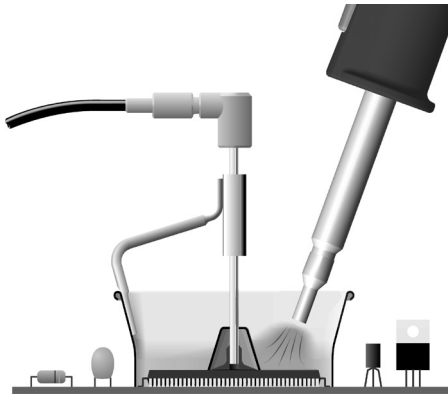
2. Hot-air melts the solder
