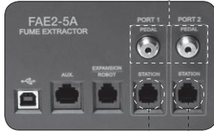
*The pedal connection takes precedence over the RJ12 connection, the equipment will only attend the Pedal port.*
