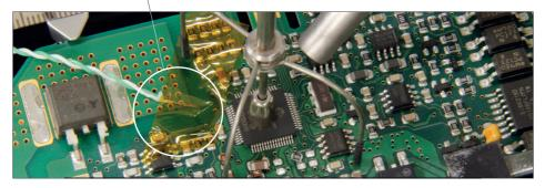
IPC\* does not recommend exceeding ramp-up rates over 3 - 4  $^{\circ}$ C / sec (5 - 7  $^{\circ}$ F / sec) so as to reduce the risk of thermal stress on the PCB.
