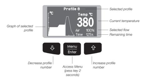
You can switch between operating modes (Manual Mode / Profile Mode) by pressing the "increase" and "decrease" keys simultaneously for 2 seconds. (Only if mode profiles is ON)
