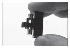
Press the new fuse into the holder and replace it in the station.
