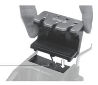
When you place the new S3-B make sure the cable fits snugly and is not pinched for a proper connection.
