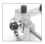
**3.** Place the guides, the rubber cups and adjust the sliding clamp knobs again.
