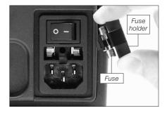
**2.** Press the new fuse into the fuse holder and replace it in the station.
