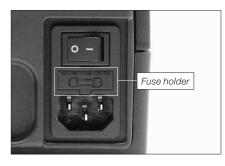
**1.** Pull off the fuse holder and remove the fuse. If necessary use a tool to lever it off.
