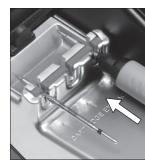
Push the cartridge into the handle to the mark\*.
