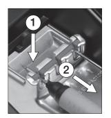
Place the cartridge in the slot as shown and pull the handle to remove it.
