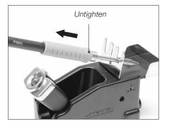
Untighten the screw. Place the Soldering Iron in the extractor and remove the cartridge.
