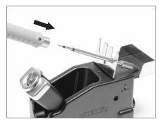
Insert the cartridge and press slightly until the mark\*
