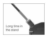
After longer periods of inactivity (pre-set to 30 min.), the power is cut off and the tool cools down to room temperature.
