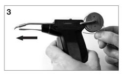
Insert the solder into its hole checking that the wire becomes straight. Pull the trigger intermittently until the solder feed system works by itself.
