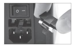
Remove the fuse by pulling the black cap. Help yourself with a lever tool if necessary.
