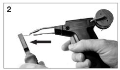
Before fitting a new reel, pull out the solder remaining inside the solder direction tube.
