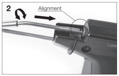
Place the new cartridge in the solder feed handle. **Important:** It is essential to insert the cartridge till the end for a good connection. Use the mark ▶ as reference.
