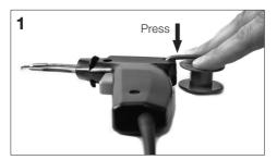
Press the empty reel to remove it and replace it with a new one.
