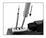
Place the handpiece on top of the new cartridge, press it down slightly and remove the handpiece from the extractor.
