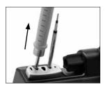
Place the handpiece in the extractor and remove the cartridge.
