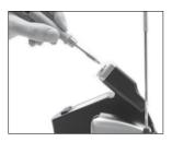
Lift tool from the stand and the tool tip will heat up to the selected temperature.
