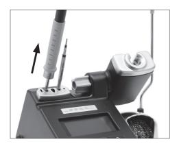
Place the handpiece in the extractor and remove the cartridge.
