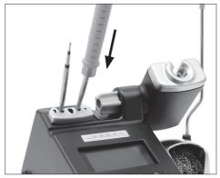
Place the handpiece on top of the new cartridge, press it slightly down and remove the handpiece from the extractor.
