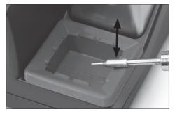
Tap smoothly the cartridge on the wiper profile to remove the excess of solder
