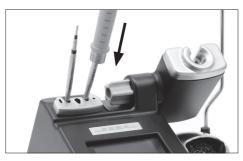
Place the handpiece on top of the new cartridge, press it slightly down and remove the handpiece from the extractor.
