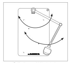
Position the arm and tighten the knobs.
