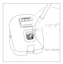
The tip cleaner is automatically switched off if the splashguard is opened during operation.
