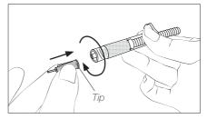
Thread the tip onto the syringe barrel.
