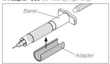
For 3cc syringes in use with DPM the enclosed adapter is needed. Assemble the adapter by clipping it onto the barrel.
