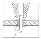
Place the tip with the component terminal in the hole.
